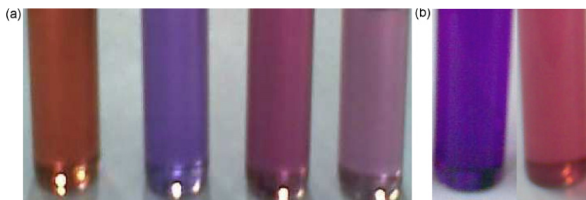
Fig. 3. Visible color changes of receptor 1 solution upon addition of 5 equivalents of each (a) anions; from left to right, receptor 1; with acetate; benzoate and formate and (b) cations; from left to right, with Cu II and Zn II .
